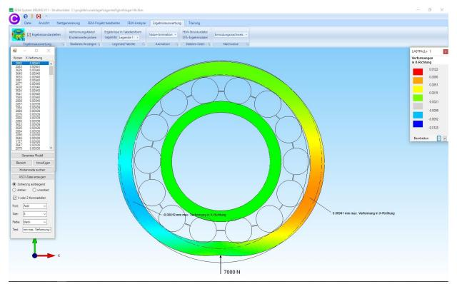
Deformations in the X direction with a deformation factor of 100
