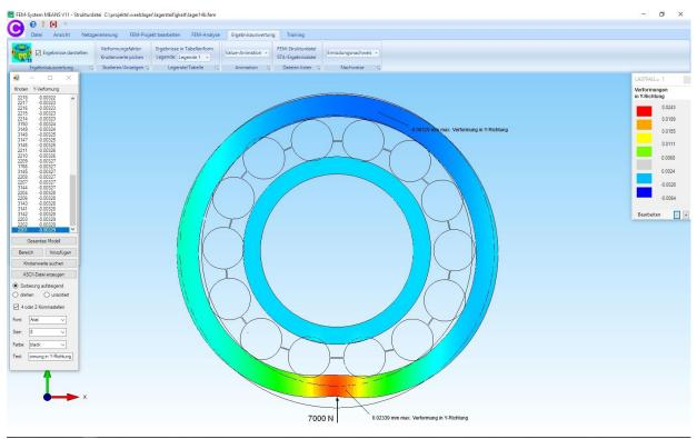
Deformations in the Y direction with a deformation factor of 100
