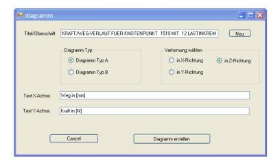
Choose "Open" and select the File "Diagram.plt" to show the displacments and the loads for node 1519 in a diagram.
