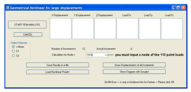
After the nonlinear Calculation select "Show Displacements of all Increments"
